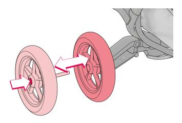
To remove a back wheel, press and hold the pushbutton (19) and pull the wheel off the axle.
