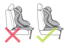
Push the release button (09) outward and position the support leg (10) so that it rests securely on the floor and the safety display shows GREEN.
