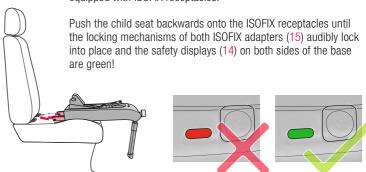
Now reinsert the seat, depending on the age of the child either in the driving direction or opposite to it (see "MOUNTING THE SEAT OPPOSITE TO THE DRIVING DIRECTION (FROM BIRTH TO 13 KG)" or "MOUNTING THE SEAT IN THE DRIVING DIRECTION (FROM 9 - 18 KG)").
