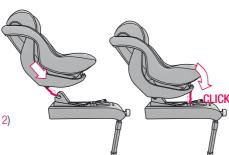
Then fold the seat forward until the front seat lock (11) audibly locks into the ISOFIX base and the safety display (07) on the top is green.
