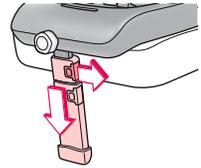
Release the control button (09) to lock the leg support in place.
