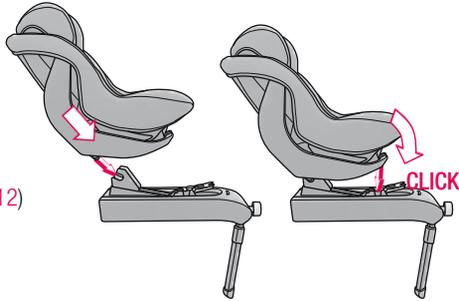
Then fold the seat forward until the front seat lock (11) audibly locks into the I-Size base and the safety display (07) on the top is green.
