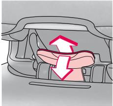
The unlocking mechanism of the seat lock (06) is at the front underneath the seat on the top of the I-Size base.
