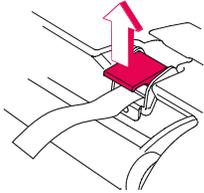
At the front of the seat under the cover there is the central adjusting device (03), which clamps the central harness (04) tight. Loosen the central adjusting device (03) by pushing the cap of the central adjusting device up and pull the harness forward (do not pull on the harness cushioning!).
