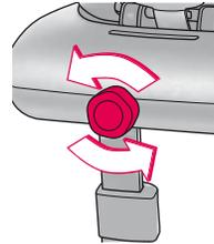
Turn the ISOFIX SYSTEM (08) control knob on the front of the CONCORD ULTIMAX I-Size base to the left until the ISOFIX adapter (15) on the reverse is fully extended.
