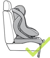
Push the release button (09) of the upper leg support adjustment outward and position the leg support (10) for it to rest securely on the floor and the safety display shows GREEN. If necessary, the lower leg support adjustment needs to be used as well.
