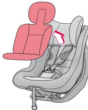
The pre-installed baby insert should be removed, if the child's height exceeds 60 cm.
