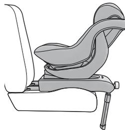
Push the child seat backwards onto the ISOFIX receptacles until the locking mechanisms of both ISOFIX adapters (15) audibly lock into place and the safety displays (14) on both adapters are green!
