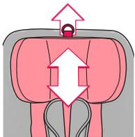
The shoulder belt guide should be situated slightly above the child's shoulder. The shoulder belt should lie in the middle between the child's neck and the outer edge of the shoulder.
