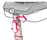
Release the control button (09) to lock the leg support in place.
