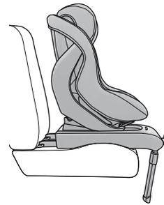
Push the child seat backwards onto the ISOFIX receptacles until the locking mechanisms of both ISOFIX adapters (15) audibly lock into place and the safety displays (14) on both adapters are green!
