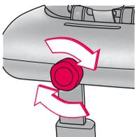
Turn the ISOFIX SYSTEM (08) control knob to the right until the ISOFIX adapter (15) is fully extended.
