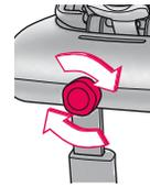
Turn the ISOFIX SYSTEM (08) control dial to the right until the CONCORD ULTIMAX lies as close/flush as possible to the back rest of the car seat.
