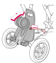
Fold down the CONCORD SLIDER and subsequently move the central hinge (04) upwards and to the left until the locking (05) on the central hinge audibly and firmly engages.
