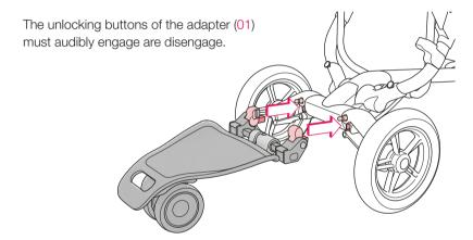
Before each journey, check to make sure that installation has been carried out correctly, the locking mechanism is closed and that the central hinge (05) is locked.
