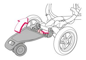
Attach the CONCORD SLIDER using the safety belt (03) previously attached to the CONCORD NEO.
