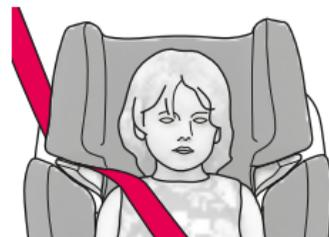
The shoulder belt guide (07) should be slightly above the top of the child's shoulder. At the same time, the shoulder belt should pass centrally between the child's neck and the outer edge of the shoulder.
