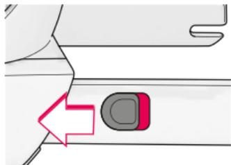
To remove the CONCORD TRANSFORMER, pull the TWINFIX button (09) forwards and move the seat fully forwards. Next, slide the locking buttons on the outer sides of the TWINFIX adapters (10) forwards until the safety indicators are red. Now pull the seat forwards and away from the ISOFIX points.
