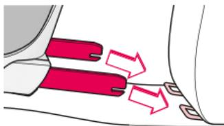
Push the child car seat back and onto the ISOFIX points until the locking mechanisms on both TWINFIX adapters (10) have clicked audibly into place and the safety indicators on both adapters are green!
